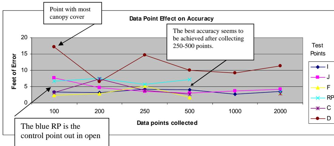
The best accuracy at the 3 test points with the most canopy cover were achieved after capturing 250 data points, with external antennas, and during optimum satellite conditions. Post processing done on all of the units, except for the Garmin 60 & 10.
